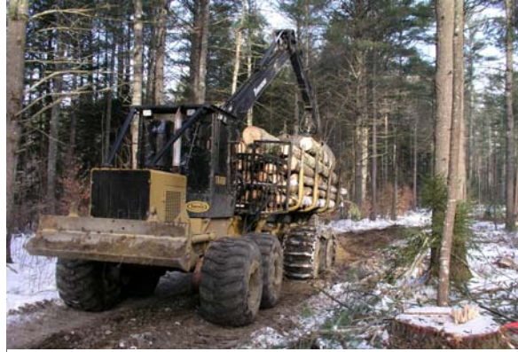
Figure 1 A forwarder bringing pulp to the yard on a timber harvest on a New Hampshire state reservation.
